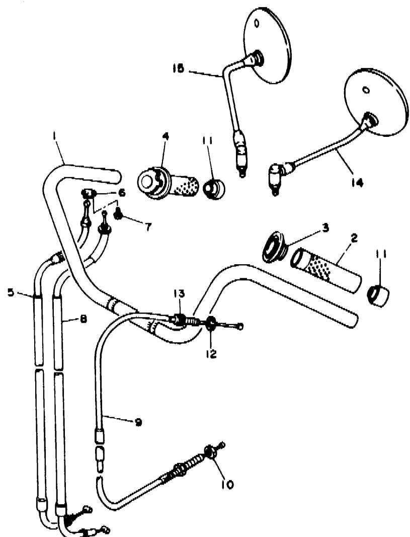
FIG. 31 STEERING HANDLE, CABLE
