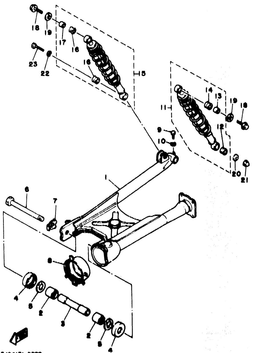
FIG. 22 REAR ARM. SUSPENSION
